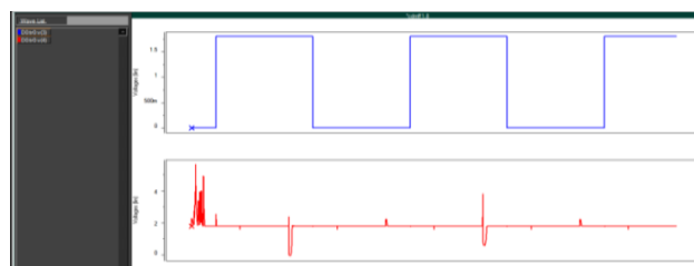
Fig.7 Conditional Data Mapping Flip Flop floating problem wave form
